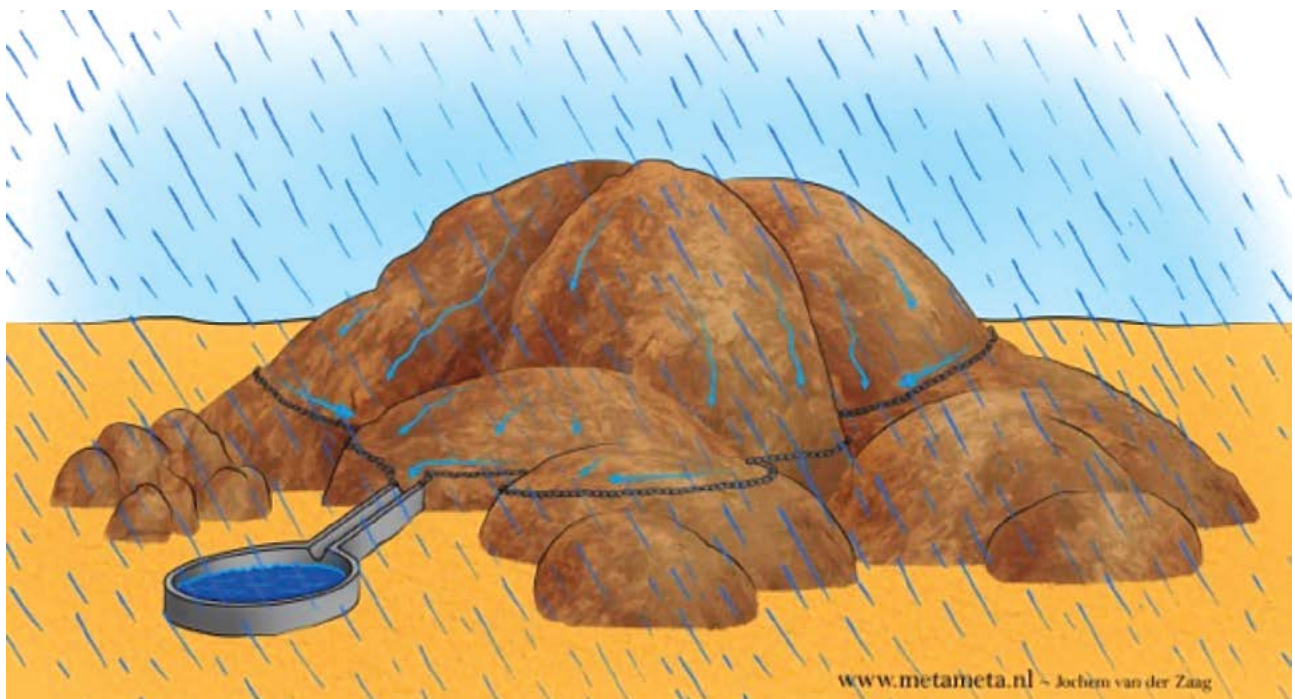
Figure 16: Rock catchments allow the capture of water (Source: MetaMeta)
